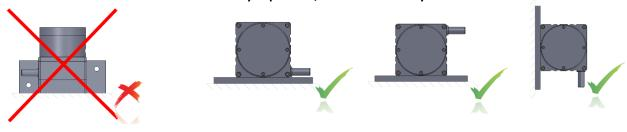
3. If there is a trickle of water (like a rain), the wire outlet must not be a drip of water upstream. If needed please use guide rollers.
